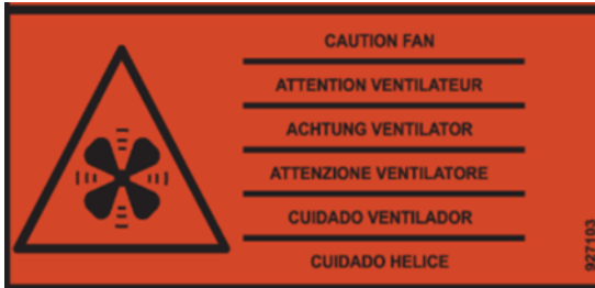
Figure 2. Fan Warning Nameplate
