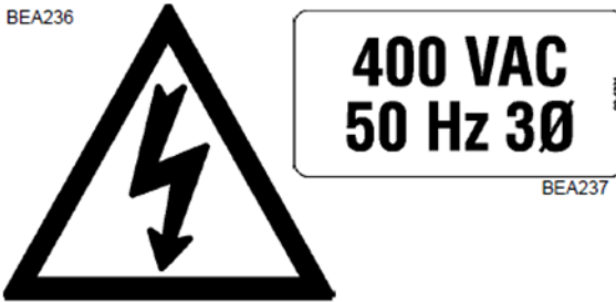
Figure 4. High Voltage Warning Nameplate
